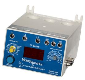
SymCom's Model 777-LR-HRG-P2 is a fully programmable electronic overload relay that is designed for resistively grounded systems. The 777-LR-HRG-P2 is recommended for monitoring and protecting any 3-phase 200-480VAC motor, used in a high resistance grounded (HRG) system, drawing 91-800 full load amps (external CTs are required). The units provide unsurpassed protection from faulty voltage and current conditions.
